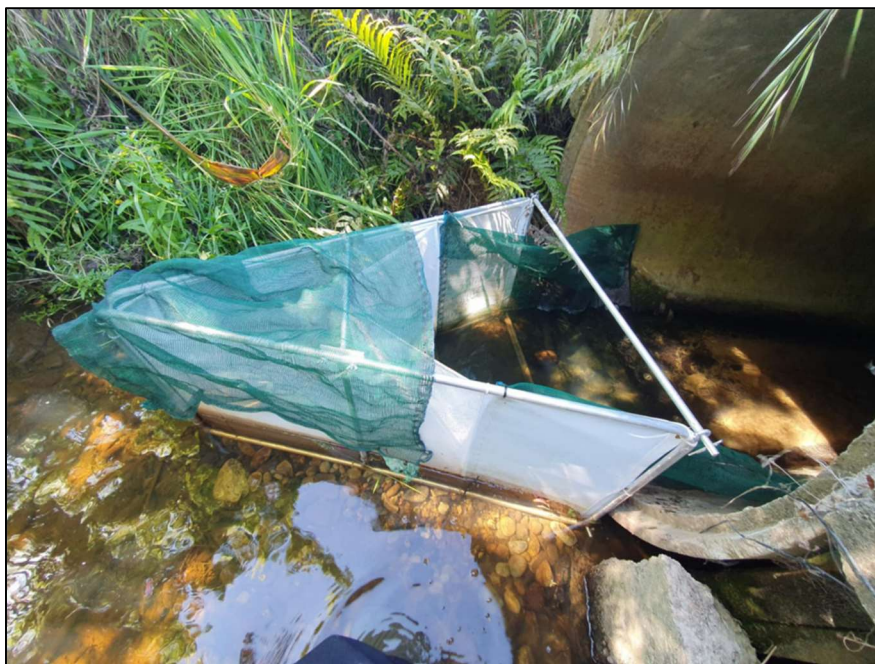
Figure 16. Inlet A-frame trap at the Williams Creek culvert.
