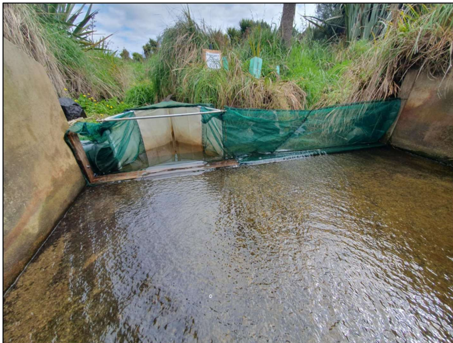
Figure 5. Inlet A-frame trap and screening wings at the Dominion Stream box culvert.
